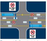
**Turn restrictions** limit left or right turns for general traffic to reduce delay for buses and other vehicles traveling along a corridor. Buses may be exempted from the restrictions.
