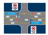
**Turn restrictions** limit left or right turns for general traffic to reduce delay for buses and other vehicles traveling along a corridor. Buses may be exempted from the restrictions.
