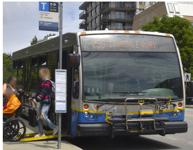
Bus bulb projects reduce the time buses spend merging into and out of traffic while also providing more room for people on the sidewalk, such as at Lonsdale Ave between 4th and 5th Streets.
