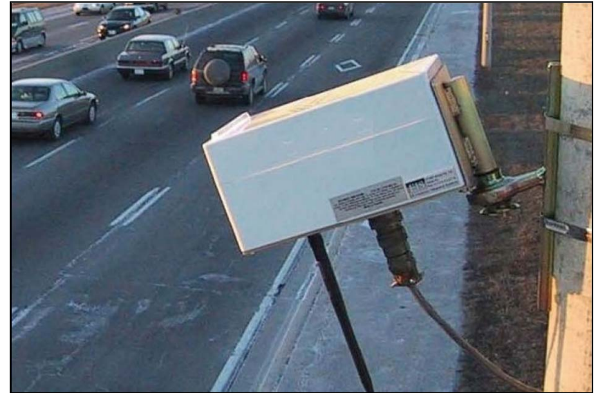
Figure 5 – RTMS Vehicle Detector
